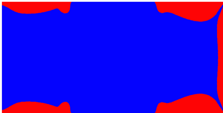
Figure 22: Plastic (red) and elastic (blue) zones in Example 2.
