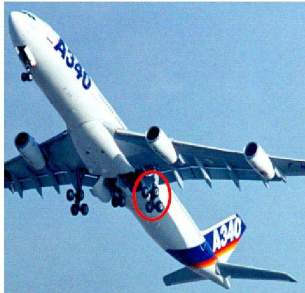
Figure 1.1: The landing gear of an aeroplane
