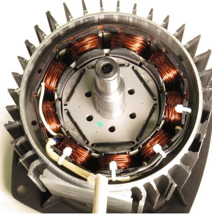
Figure 2.1: Interior permanent magnet synchronous motor as produced by Hanning Elektro-Werke GmbH & Co KG. Photo credit: LCM GmbH.
